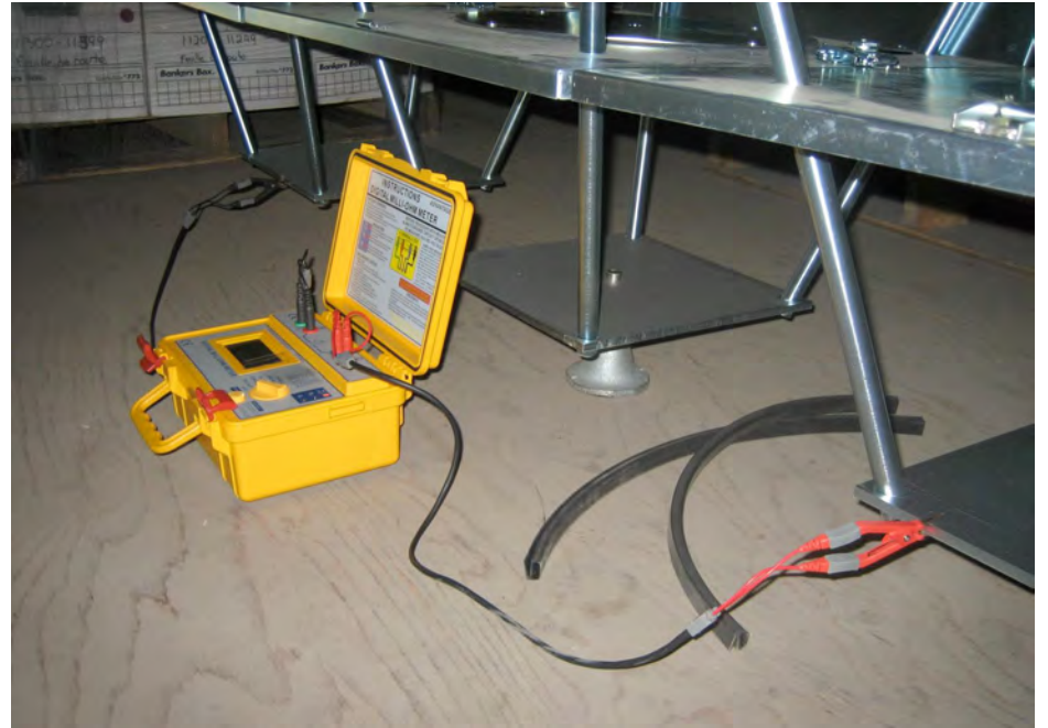
Pic. 8-Edge of Mod. 1 Bottom Supt. to Edge of Mod. 3 Bottom Supt.-Read. 2.3 mOhm
