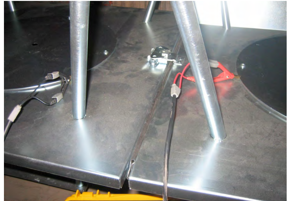
Pic. 11-Edge of Mod. 1 Cover Plate to Edge of Mod. 3 Cover Plate-Reading 2.4mOhm
