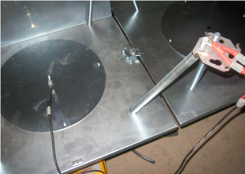
Pic. 6- Center of Module to Top Panel Support Lug-Reading .7 mOhm
